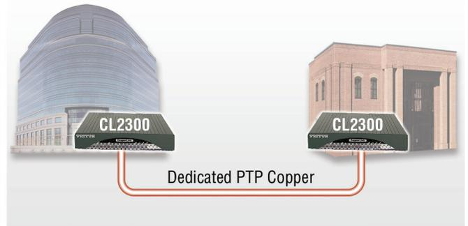
When interconnecting sites on a corporate campus, buildings and network devices often lie beyond reach of a standard Ethernet segment. Now, you can use existing copper network infrastructure to connect remote LANs or devices across longer distances and at higher speeds than previously thought possible.
