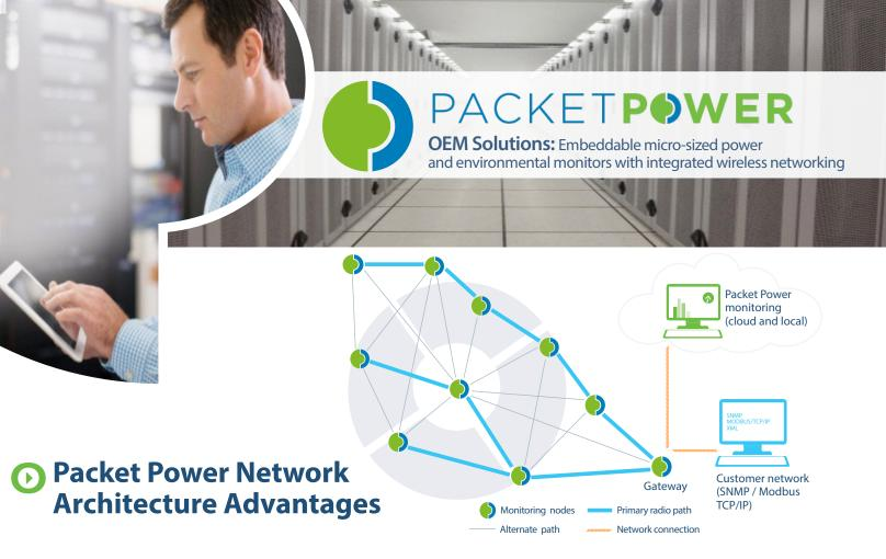
The convenience of wireless with the reliability of a wired network. Packet Power's self configuring mesh network delivers all the advantages of wireless connectivity while eliminating the traditional difficulties associated with wireless propagation and system configuration. Using a "mesh topology," the system routes data from one
