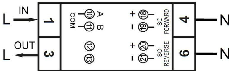
*When connecting the meter through a serial converter (RS485) for testing, please be aware that because of not implementing the complete Modbus infrastructure, there will be a need to put an additional resistor (120 ohms/ 0.25 watts) across the terminals (10 & 11) on the meter side.*
