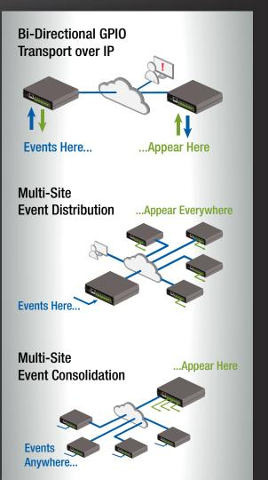
Transport digital I/O across Ethernet networks with IP protocols. Any changes in status appear at the other end of the network as relay outputs. Multiple iPIO units can communicate to broadcast GPIO status to many locations, or consolidate status at a single point.
