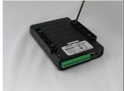
Install the DIN rail clips using the black screws as shown
