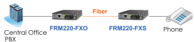
Figure 2 : Voice Transmission from 2km to 120km over fiber
