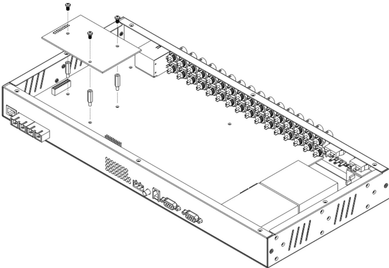
Figure 2-8 : SNMP module card Removal / Replacement
