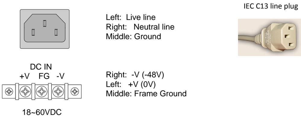
Figure 2-2 : Supply connections, AC/DC model shown
