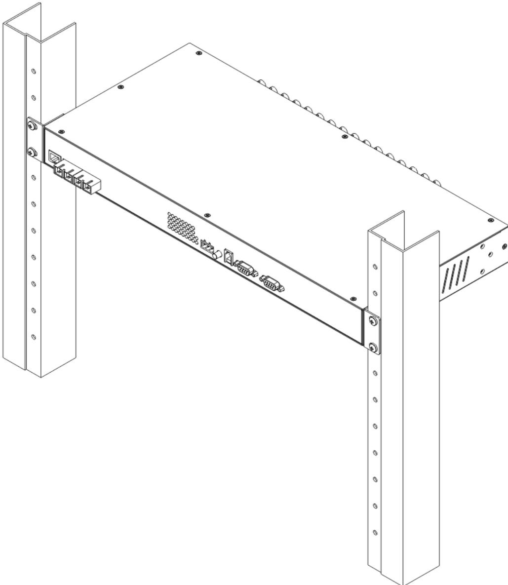
Figure 2-1 : Rack mount Installation of the **Fiber Multiplexer**
