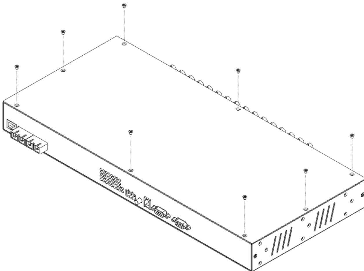
Figure 2-7 : Top cover removal (while out of service)
