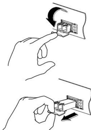
Figure 2-5 : Optical Interface Removal / Replacement (while in service)
