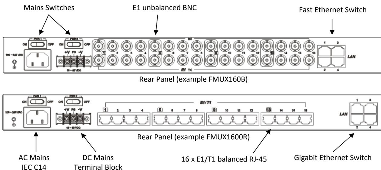
Figure 2-3 : Rear Panel Connections
