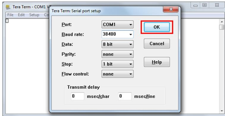
Figure 3-1 TeraTerm Pro port settings for Fiber Multiplexer
