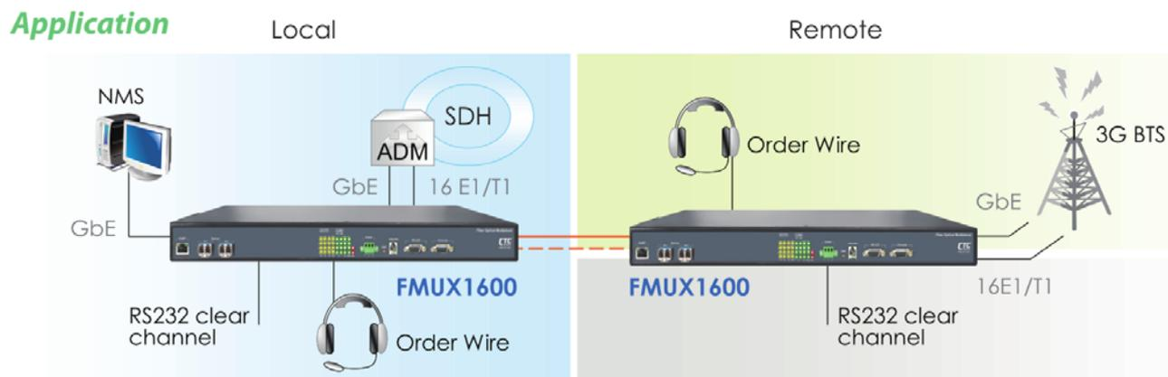
Figure 1-2 : Typical Point-to-Point Application of *Fiber Multiplexer*
