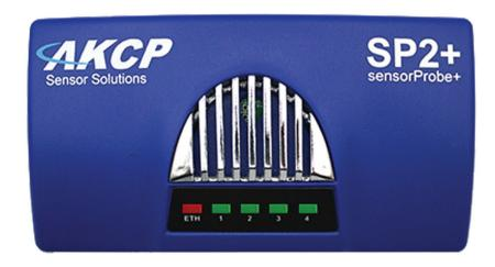
SP2+ comes with 4x intelligent sensor ports that can be used to connect a wide range of AKCP sensors, as well as support for our new range of smart sensors such as thermal maps and LCD displays.
