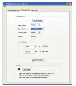
TT336 Model software allows you to configure transmitters offline, save the file, and download into units later, at your convenience.
