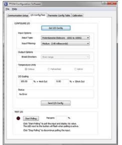
TT234 Model software allows you to configure transmitters offline, save the file, and download into units later, at your convenience.
