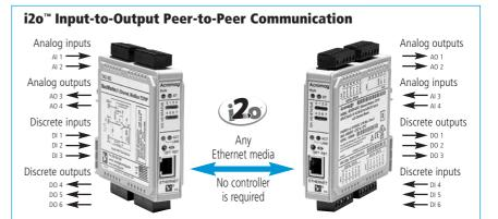
Acromag's i2o technology allows modules to talk directly to another module across any Ethernet media without a PLC, PC, or other controller in between. Input channels on one module can write to output channels on a remote module.
