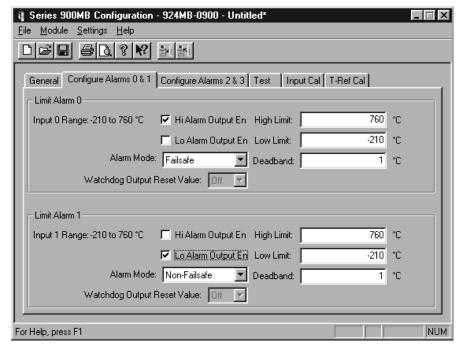
Limit alarms are easy to configure with fill-in-the-blank fields in engineering units for high/low alarm setpoints.
