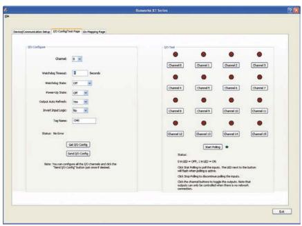
BusWorks XT software (download free from www.acromag.com) allows you to configure transmitters offline with USB, save the file, and download settings into units later, at your convenience.
