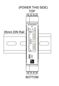
TILT MODULE UPWARD TOWARDS RAIL AND HOOK ONTO UPPER LIP OF RAIL. ROTATE MODULE DOWNWARD TO ENGAGE SPRING CLIP ONTO LOWER LIP OF RAIL.
