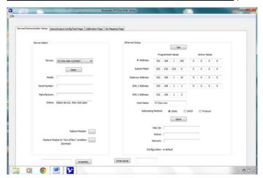
Once you have selected a device, click the **[Open]** button to open communication with the unit and the screen will fill out similar to the following (the selected unit's Model, Serial Number, Manufacturer, and a USB connection status message will be displayed as shown in the screen below):
