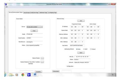
The Device Communication Setup screen is split into two parts: Device Select & Ethernet Setup.
