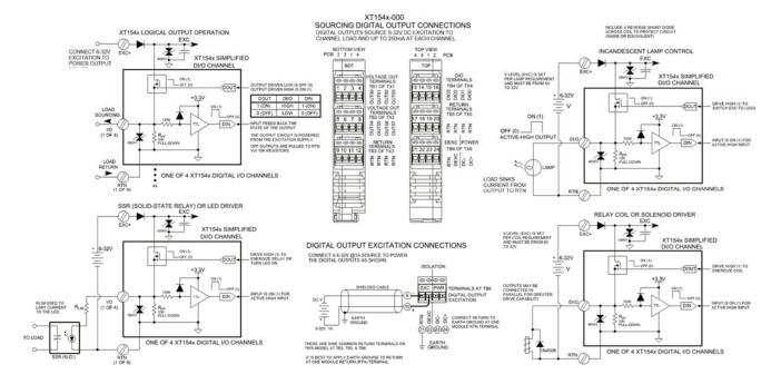
**NOTE:** You must connect digital EXC to a voltage source from 6 to 32VDC in order to operate the digital outputs, as the sourcing digital output driver is also powered from the excitation supply.
