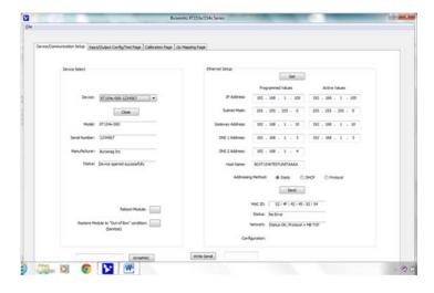
An **IP Address** (Internet Protocol Address) is a unique identification number for any host (this module) on any Ethernet/IP network (including the internet). It uniquely defines one host from all other computers (hosts) on the Internet. The IP address is made up of four octets (8 bits), each octet having a value between 0-255 (00H-FFH). It is expressed here in decimal form, with a period between octets.
