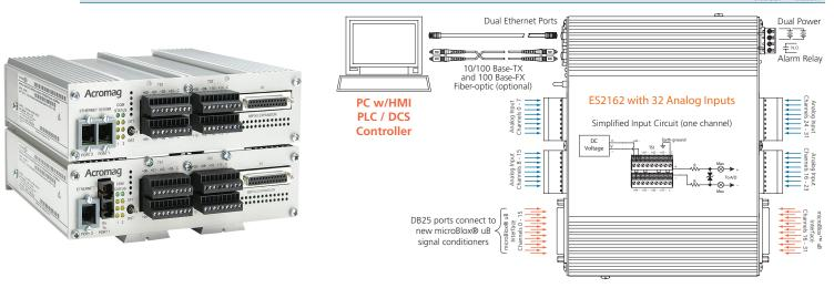
32-channel differential analog voltage input with uB interface
