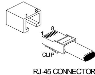
The Ethernet port of this unit is wired MDI-X by default, but includes automatic crossover (the Ethernet port of your PC is typically wired MDI). Thus, you can use either a straight-through or crossover cable to connect this device directly to a PC, Ethernet switch, or another unit.
