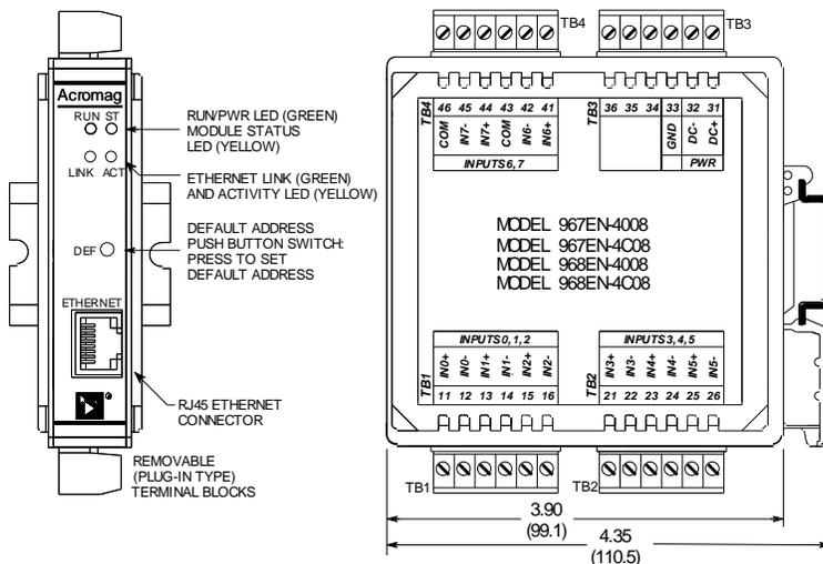
The front panel DFT push-button is used to toggle the module into or out of Default Mode. In Default Communication Mode, the module assumes a fixed static IP address of "128.1.1.100", a default subnet mask of "255.255.255.0", a default username of "User", and a default password of "password". To activate, depress the DFT button for 5 seconds, until the ST LED blinks on/off slowly. To disable, depress the DFT button for 5 seconds or until the ST LED stops blinking.
